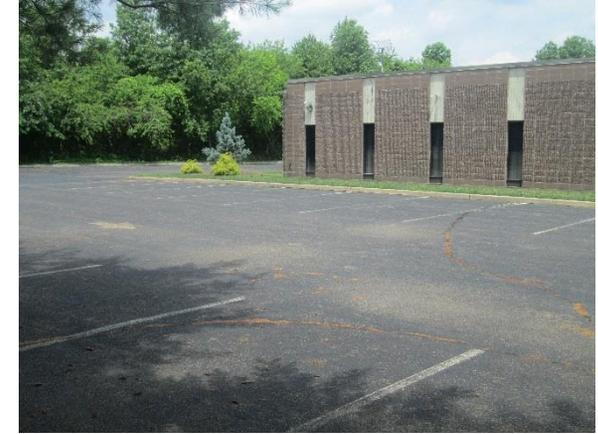
Parking lot runoff can be captured and infiltrated by installing porous asphalt in parking spaces around the building. A bioretention system can be installed on the eastern side of the site to manage additional parking lot runoff. A preliminary soil assessment suggests that the soils have suitable drainage characteristics for green infrastructure.
