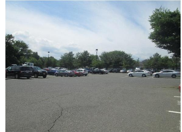
Porous asphalt can be installed along three strips of parking spots to capture and infiltrate parking lot runoff. A bioretention system can also be installed off of the southern side of the building to capture, treat, and infiltrate additional stormwater. A preliminary soil assessment suggests that the soils have suitable drainage characteristics for green infrastructure.
